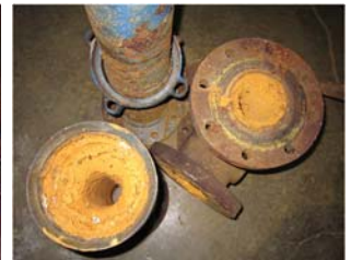
Above is a picture of the state of the existing corroded pipe.
